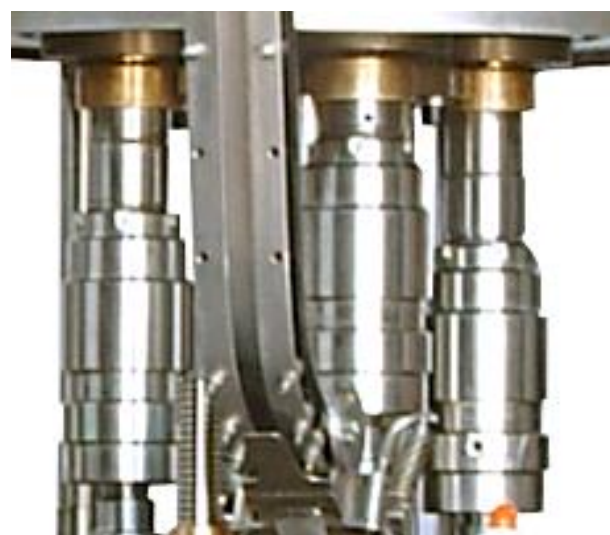
Capping heads equipped with Magnetic clutch
